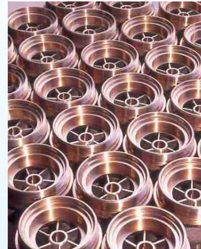
The heavy duty phosphor bronze and stainless steel construction of Southern Cross “NA” Electric Submersible Borehole Pumps, combined with the excellence of hydraulic design and component manufacture, provides exceptional reliability and ongoing operating efficiency for the most demanding borehole pumping applications and where continuity of supply is essential.
